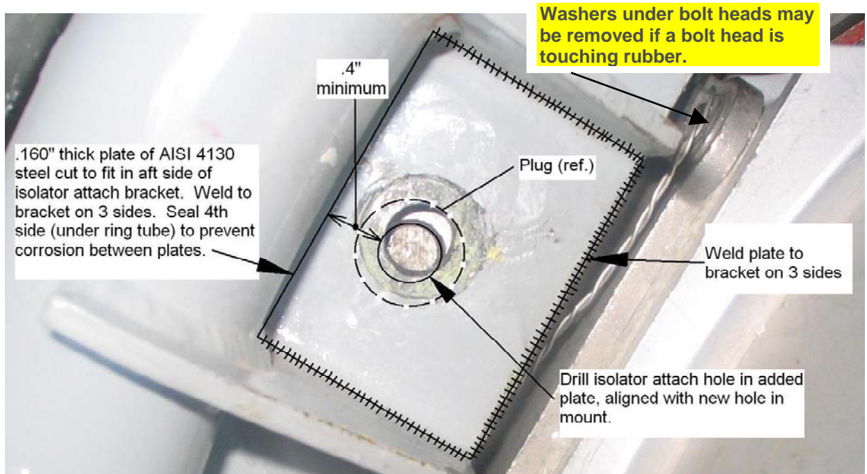
Figure 3: Plate Installation
